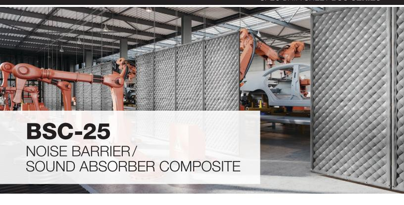
The barrier septum configuration of Sound Seal's **BSC-25** product offers the benefits of both a sound absorber and noise barrier. Each curtain is custom fabricated to include a non-reinforced 1-lb psf loaded vinyl noise barrier sandwiched between two layers of 1" thick acoustical fiberglass sound absorbers. Each panel is finished with a quilted, vinyl-coated-fiberglass-cloth facing, grommets across the top, and vertical-mating Velcro along the edges for easy installation.
