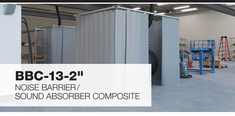
The configuration of Sound Seal's **BBC-13-2"** product offers the benefits of both a sound absorber and noise barrier. Each curtain is custom fabricated to include a reinforced 1-lb psf loaded vinyl noise barrier bonded to a 2" thick layer of fiberglass that is quilted with a vinyl-coated-fiberglass-cloth facing. Each is finished with grommets across the top, and vertical-mating Velcro along the edges for easy installation.
